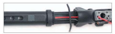
17. For models with stock tube: Pass the Control Unit and the Data Wire through the stock tube. Place the wires in the wire channel of the stock tube, keeping the data wire protected under the red and black wires as shown in the picture above. Very carefully slide the stock tube into the receiver while watching that the wires stay in the wire channel. If the stock tube does not slide in easily refer to the last NOTE above.
