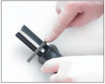
**15**. Pass the Control Unit and the Data Wire through the opening in the pack of the lower receiver as shown on the picture.
