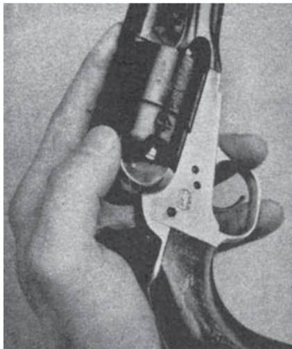
Place cap on each loaded chamber.
