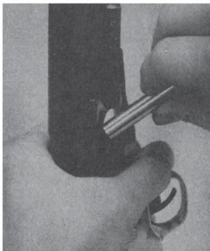
Pour a measured charge into chamber.
